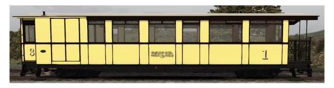
The brake coaches, numbers 1 and 3, were composites with first class at the veranda end and entry to third class through the guards compartment.
