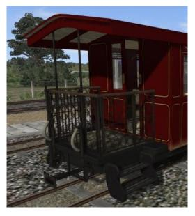
The original coaches had vacuum brakes but these models also have air brakes as most of the NG stock has either air or vacuum brakes and so these models will work with either. Each coach was fitted with two pipes to enable them to connect to the low pipes on the transporter wagons. I have not modelled these connecting as it was too hard to do ! All of the coaches also have handbrakes. The handbrakes at the end of each coach are not animated but can be turned on using the F3/F4 dashboards.
